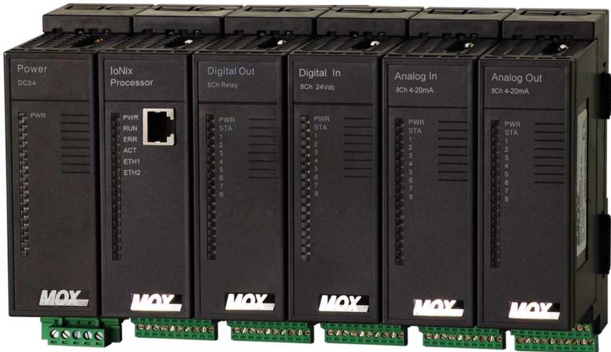
Figure 22 Rack Base I/O Modules Connected to MOX IoNix
